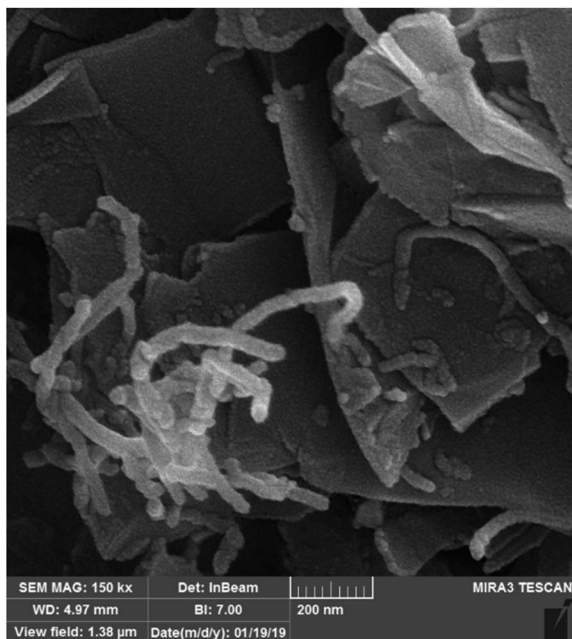
Fig. 8 An FESEM image of nano-MgO@CNT@Gr after five sequential COP experiments.
