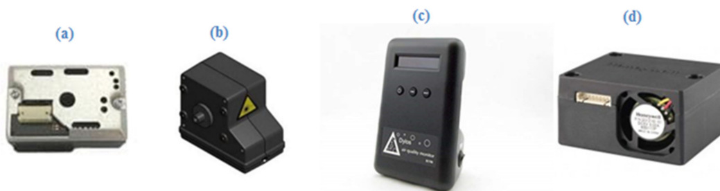
Figure 2. The COTS sensors that were used for the measurements: (a) Sharp-GP2Y1030AU0F; (b) OPC-N3; (c) Dylos DC1700; (d) Honeywell HPMA115S0-XXX.
