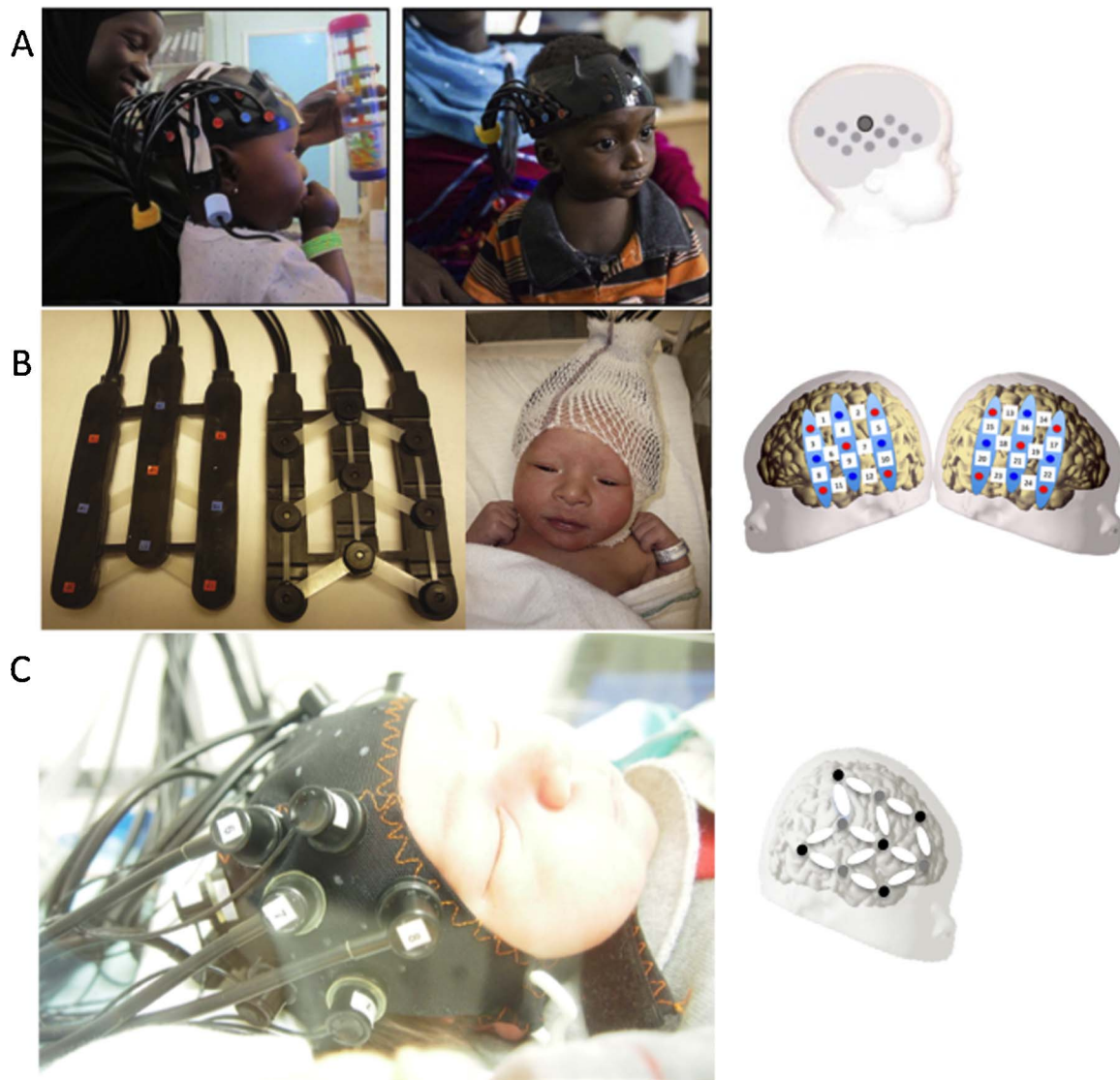
Fig. 2. Pictures of different fNIRS headgears and their respective approximate channel locations. A: The UCL system (adapted from Lloyd-Fox et al., 2018). B: The Hitachi ETG-4000 system (adapted from May et al., 2011). C: The NIRx NIRScout system as used in our laboratory.
