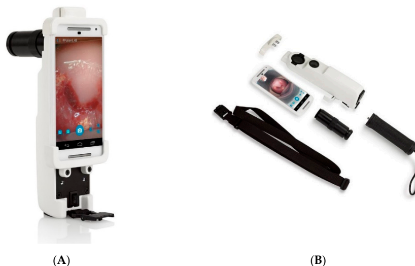
Figure 1. Photos of the Enhanced Visual Assessment (EVA) System's mobile colposcope, either assembled (A), or split into its various components (B).
