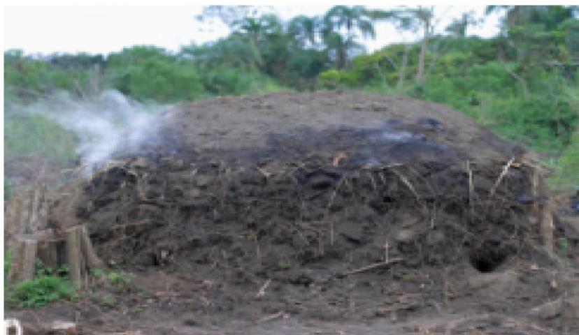
Fig. 8. Kiln adjusting itself to insufficient oxygen supply.
