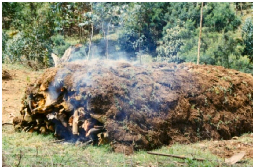
Fig. 7. Fire starting at the ignition point.
