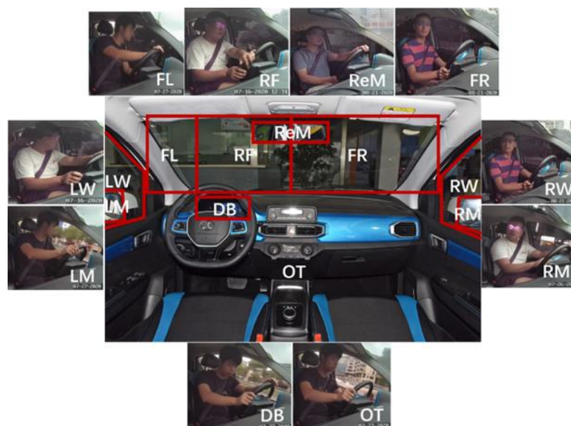
Figure 4. The specific locations of AOIs determined by the drivers' views and the corresponding photographs. RF refers to right front, FL refers to front-left, FR refers to front-right, LW refers to left window, LM refers to left mirror, RW refers to right window, RM refers to right mirror, ReM refers to rearview mirror, DB refers to dashboard and OT refers to others.
