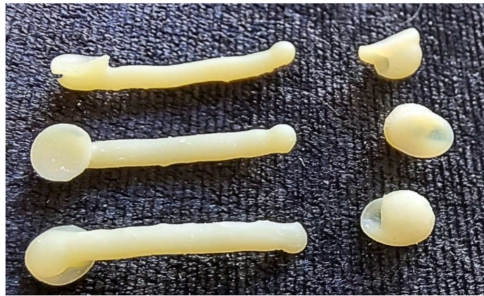
Figure 14. Three clones of a 3D printed distalizer from material Denture Teeth, shade A2.
