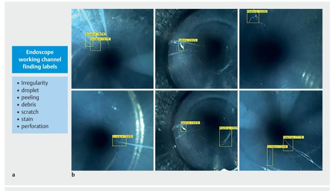
**Fig.1** a List of working channel finding labels included in the AI algorithm. **b** Sample images of deep learning algorithm-detected findings within endoscope working channels. A square depicts the finding, a label is applied to the finding and a percentage certainty is associated with the finding.
