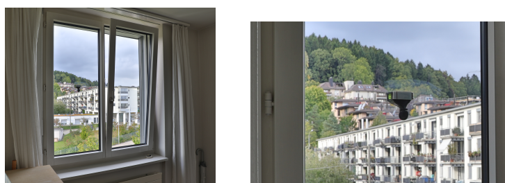
Figure 1. (Left) An example of a typical window with two sashes in a tilted position. The Noise Sentry is mounted on the left side, in the middle of the window pane; (Right) Close-up showing the Noise Sentry mounted on the window.
