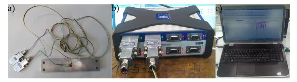
**Figure 6.** Measurement of deformations using the strain gauge method: (**a**) sample with connected SCMSG120 adapters, (**b**) HBM 1-MX840A amplifier, (**c**) computer with CatmanEasy V35.1 DAQ Project software.
