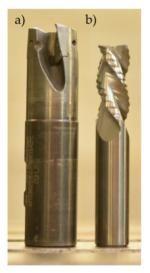
Figure 4. Tools used: (a) Kennametal indexable milling cutter, (b) Sandvik monolithic milling cutter.
