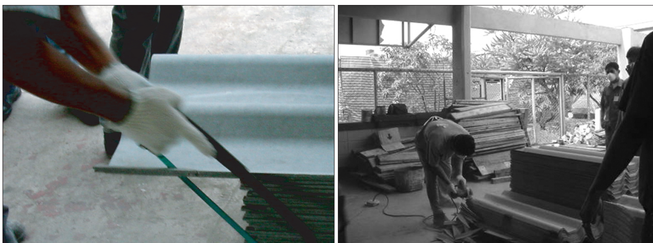
Fig. 2. Hand saw and motor saw mitering.
