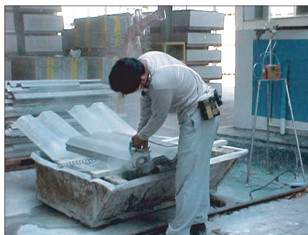
Fig. 4. Motor saw mitering.
