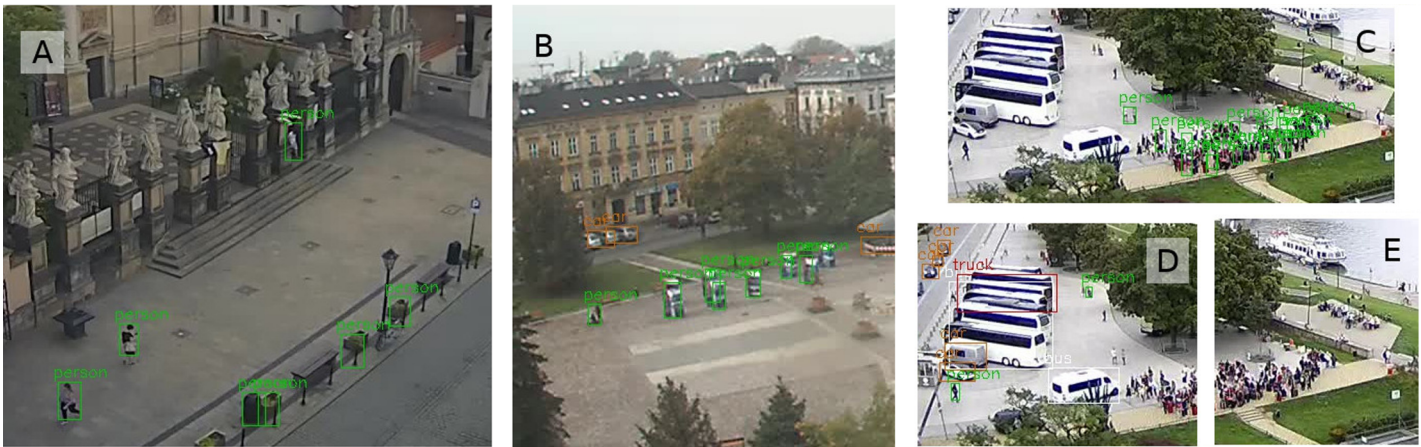
Figure 8 The biggest difference in pedestrian detection for three webcams—less pedestrians from YOLO tiled method. Error assigning class: (A) trashcan from Grodzka (bottom right), (B) advertisement display from Podgorze (only one real person was detected). Better detection of people in crowd from Wawel webcam (C) by YOLO compared to (D) and (E) YOLO tiled method. Photo credit: www.webcamera.pl .
