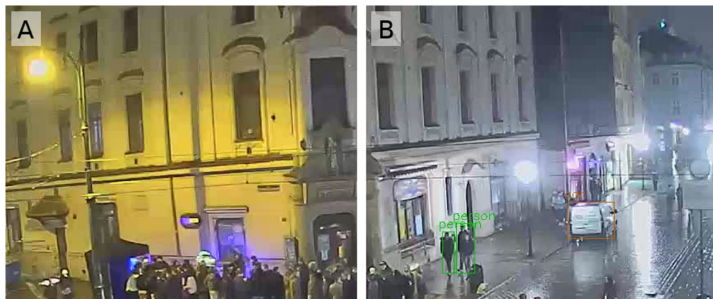
Figure 3 The upper left two tiles from the split image (Fig. 2). Pedestrians (A) undetected and (B) detected by YOLO tiled method. Photo credit: www.webcamera.pl .
