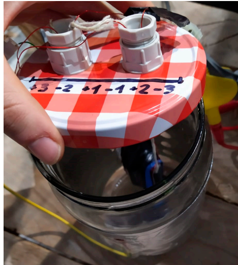
Figure 9. Two-liter container with the fluid core double coil sensor.
