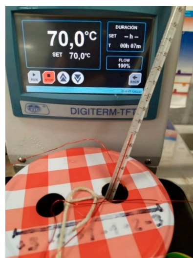
Figure 10. Controlled temperature of the dissolution of oil and water at 70 °C.
