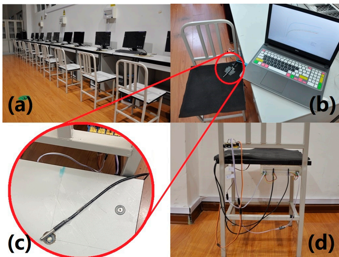
Figure 1. System construction of temperature measurement with temperature probe under the left ischial tuberosity and IRs directly beneath the cushion at the same location: (a) a perspective view of the research room with test chairs and computers; (b) top view of the experimental chair installed with 18B20 temperature probe (a water-proof metal cylinder which does not appear to significantly affect sitting comfort in asymptomatic users [19]) fastened onto the foam cushion by transparent tape; (c) IRs embedded in the wooden chair (to better illustrate the location of the IRs with respect to the temperature probe, the foam cushion has been removed); (d) rear view of the chair illustrating the data acquisition and data transmission elements.
