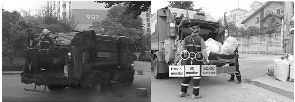
Fig 1. Photographs of municipal household waste-collecting activities. Left: Riding on the rear of a truck. Right: Collecting MHW with samplers mounted.
