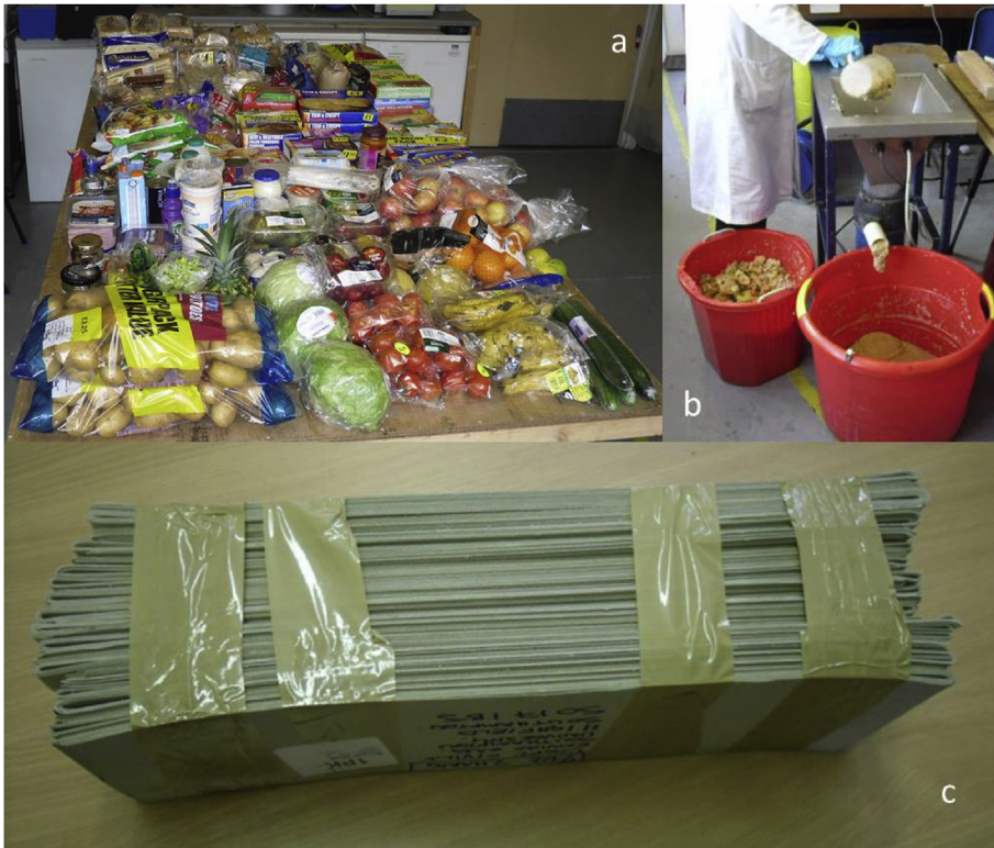
Fig. 10. Feedstock materials: (a) Materials purchased for SFW, (b) preparation of SFW by maceration, (c) unprinted card packaging also used in the mixed feed prepared for the trial.
