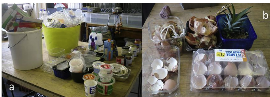
Fig. 1. Items rejected during SFW preparation: (a) Packaging materials, (b) Materials not put through macerator.
