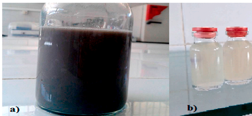
Fig. 10. Tannery effluent before (a) and after (b) adsorption onto fly ash using batch experiment.
