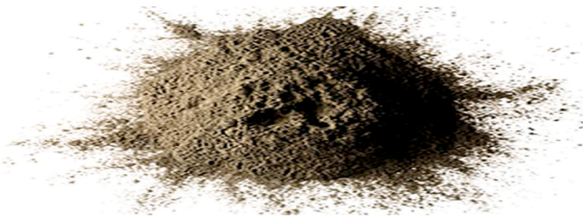
Fig. 1. Macroscopic aspect of fly ash collected from JLEC Company ELjadida, Morocco.
