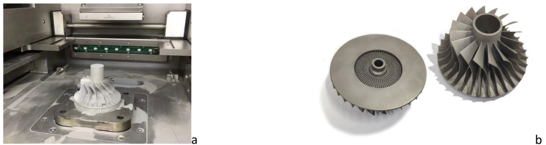
Figure 8. The unfinished lattice impeller (Support and base plate is not removed) and the finished lattice impeller || (a) The unfinished one; (b) The finished one.
