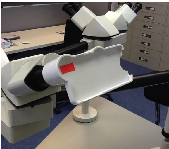
Figure 1 Smartphone adaptor attached to a microscope eyepiece to capture images for sharing on the video conferencing platform.
