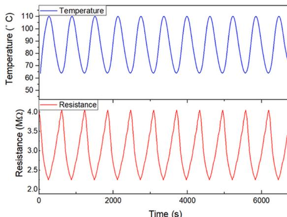
**Fig. 4.** Cyclic temperature and resistance behavior of EIL.
