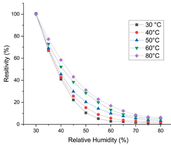
Fig. 6. The response to humidity of the sensor at different temperature.
