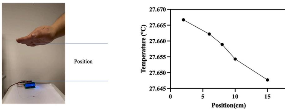
Fig. 8. The response of the sensor to hand movement.
