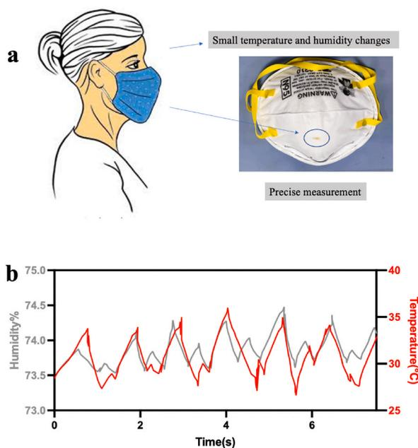
Fig. 10. (a)Schematic and photo of the breath sensor. (b) Breath testing results.
