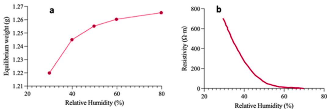
Fig. 5. (a) The equilibrium weight with the increase of humidity at room temperature. (b) The resistivity versus humidity curve of the sensor at room temperature.
