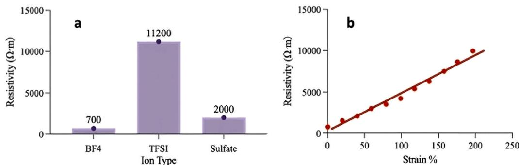
Fig. 2. (a)The resistivity of HEA ionogels with different ionic liquid. (b)Strain-resistivity curve of the material.
