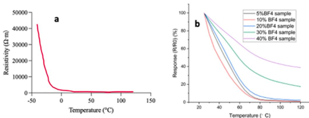
**Fig. 3.** (a) The upper and lower limit temperature sensing range of EIL. (b) The response to temperature of sample with different EMI-BF4 concentration.
