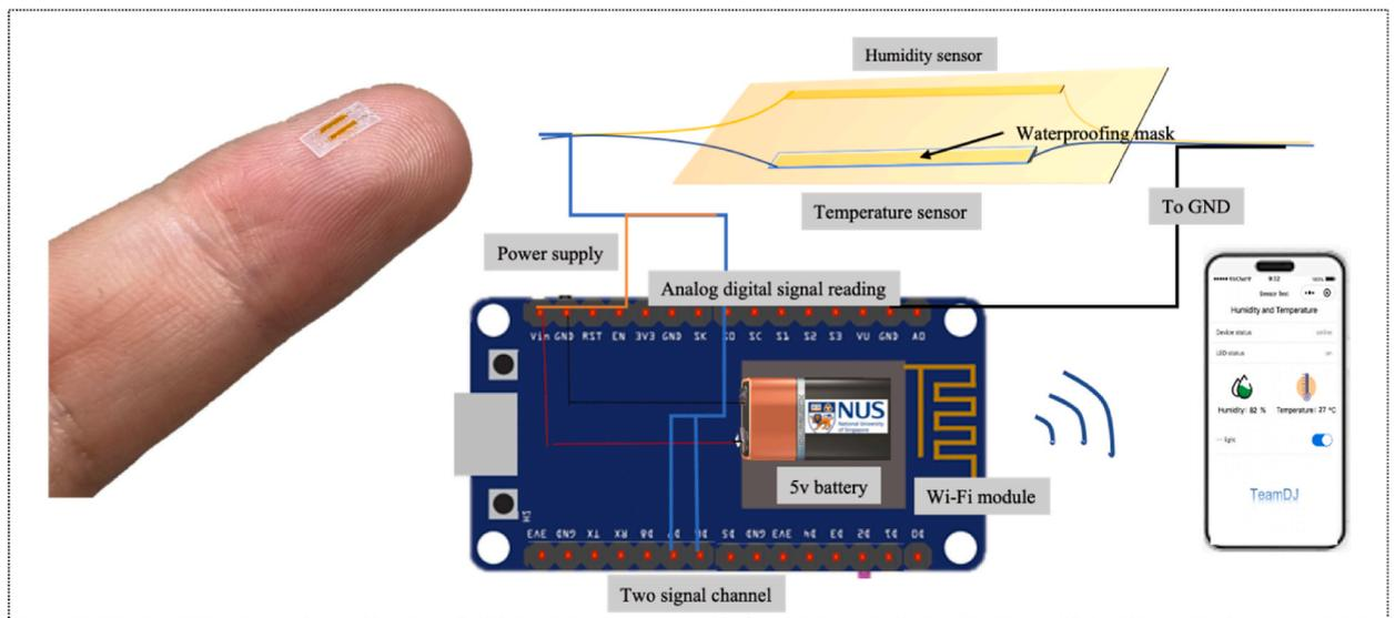
Fig. 7. Schematic and photo of the bimodal sensor.
