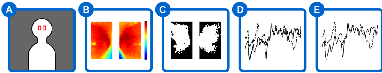
Figure 3. Mean temperature time series extraction procedure. A: The left and right periorbital regions are tracked from an initial reference frame to the end of the trial. B: The result of the tracking process is a pair of thermal videos, each showing one of the two periorbital regions (shown here with false colouring). C: For each frame of each periorbital's video, the temperature pixels are sorted from coolest to warmest and the warmest 50% of the pixels are identified. Note that the majority of the pixels on the border of the tracking region are not in the warmest 50%. D: For each frame, the mean of the 50% warmest pixels is taken for each periorbital region to generate a mean temperature time series for each periorbital region. E: The mean temperature time series is low-pass filtered to remove residual noise due to minor tracking fluctuations and thermal camera noise.
