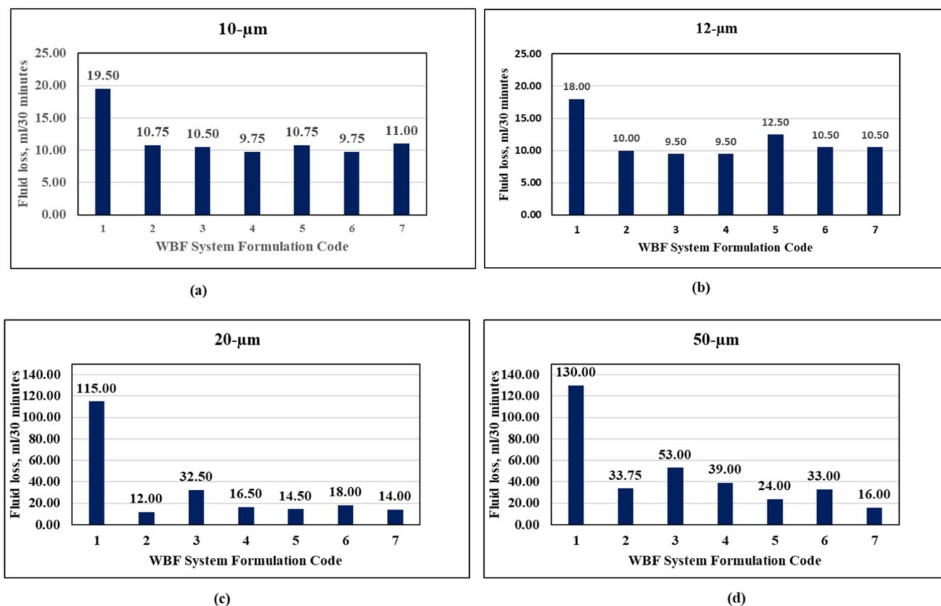
Figure 5. HPHT FL characteristics of the SMF-based fluid against (a) 10  $\mu\text{m}$  ceramic disc, (b) 12  $\mu\text{m}$  ceramic disc, (c) 20  $\mu\text{m}$  ceramic disc, and (d) 50  $\mu\text{m}$  ceramic disc under the testing conditions of 190 °F and 300 psi.
