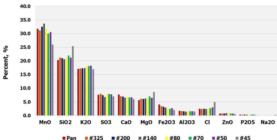
Figure 2. Elemental analysis describing the composition of the SMF-retained samples on each sieve.
