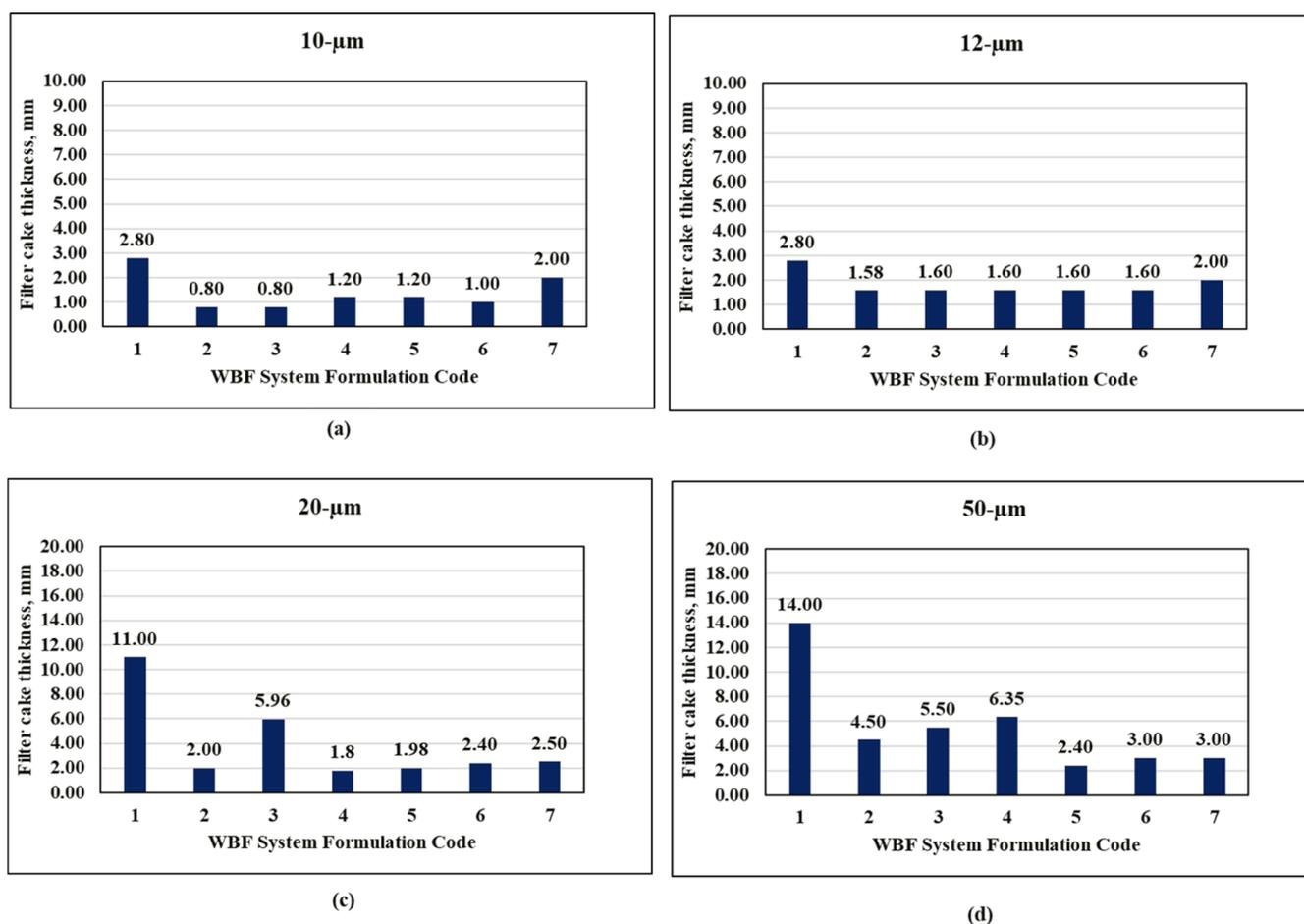
**Figure 6.** Evaluation of HPHT FC thickness for the WBF system against (a) 10, (b) 12, (c) 20, and (d) 50  $\mu\text{m}$  ceramic discs under the testing conditions of 190  $^{\circ}\text{F}$  and 300 psi.
