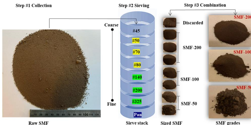
**Figure 1.** Processing steps of “raw” SMF waste material into SMF grades.
