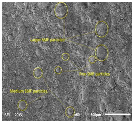
**Figure 8.** SEM photomicrograph of FC generated from the WBF-SMF system at a resolution of 500  $\mu\text{m}$ .
