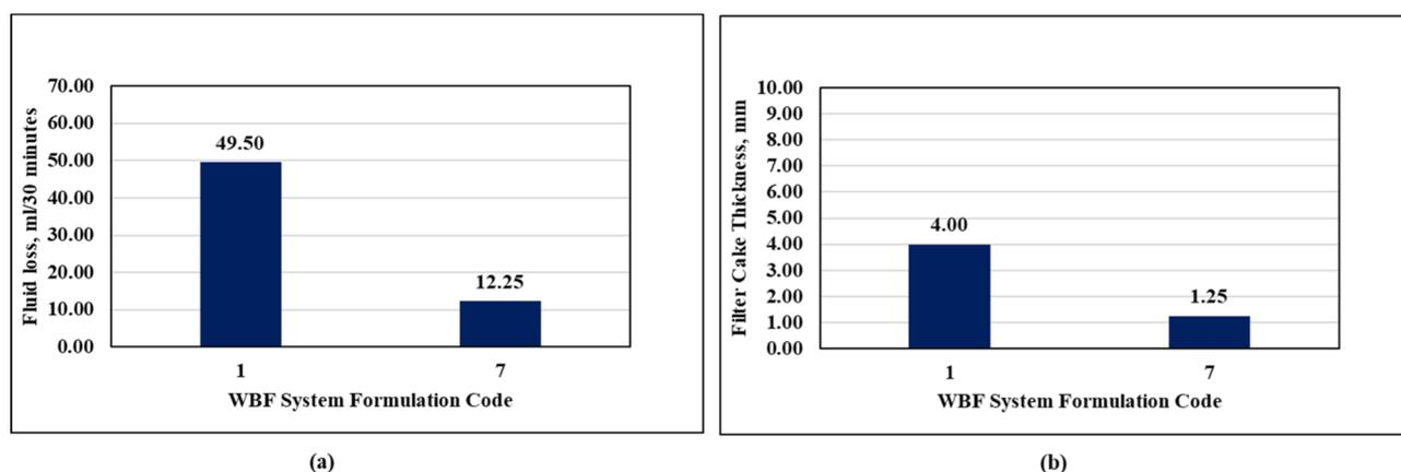
**Figure 7.** HPHT FL (a) and FC thickness (b) of formulation code 7 and formulation code 1 with 1.5 ppb of PAC tested against the 50  $\mu\text{m}$  ceramic disc.
