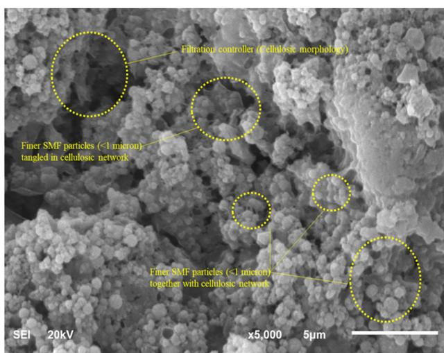
**Figure 9.** SEM photomicrograph of FC generated from the WBF-SMF system at a resolution of 5  $\mu\text{m}$ .
