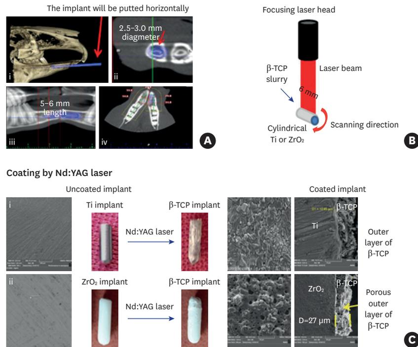
**Figure 1.** (A) Cone-beam computed tomographic images assessing the required size of the implant when it will be placed horizontally, i) 3-dimensional X-ray lateral view, ii) cross-sectional view, iii) lateral view, iv) occlusal view (B) Schematic drawing of the laser coating process for cylindrical implants, (C) FESEM images of the topography and cross-section substrate i) at the Ti-β-TCP interface area, ii) at the ZrO<sub>2</sub>-β-TCP interface. β-TCP: beta-tricalcium phosphate.
