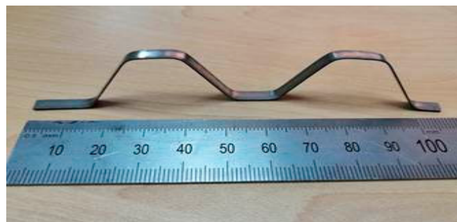
Figure 3. Monomer of NiTi SMA bracket.
