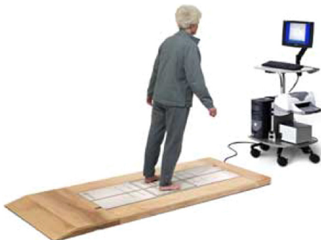
Fig. 2. Patient performing a test on a stabilometric platform.
