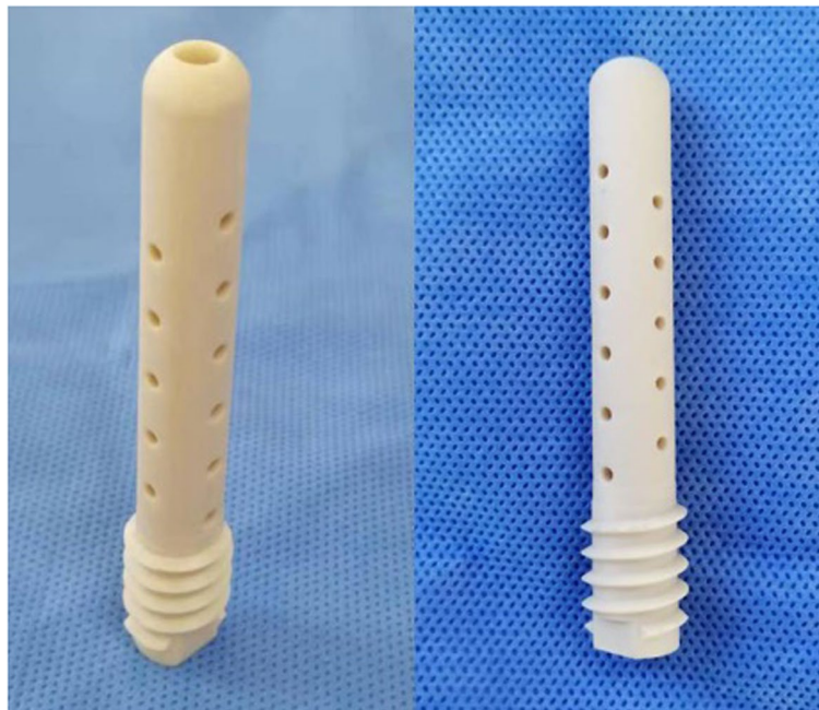
Fig. 2 The nano-hydroxyapatite/polyamide-66 (n-HA/PA66) support rod (authorization number: CF180936, hollow cylinder, 10-mm outer diameter, 4-mm inner diameter)
