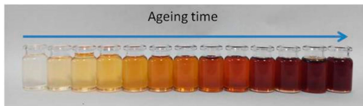
Figure 2. Change in the lubricant visible spectrum due to degradation.
