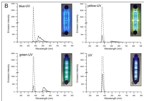
**Figure 1.** Overview of a multimodal electric trap used in field experiments (**A**). Emission intensity of single lamps emitting blue-UV, green-UV, yellow-UV, or UV only wavelengths were evaluated in laboratory conditions and are reported in arbitrary scale (**B**). For each combination of lamp and plastic grid, the emitted radiation flux was measured at close contact (continuous line) or at 2 cm distance (dashed line).
