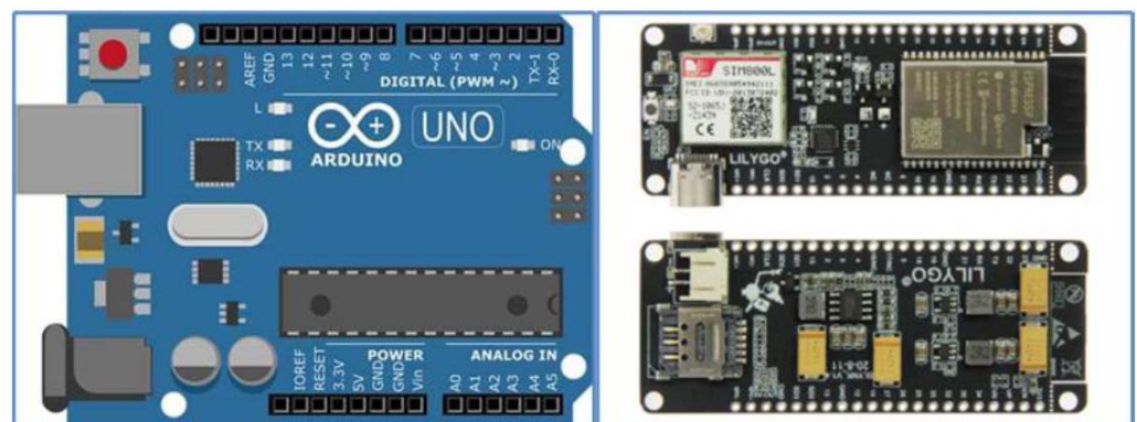
Figure 2. Arduino UNO and LilyGO TTGO V1.4 module.
