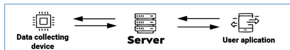
Figure 10. Simplified communication scheme of the data collection system.
