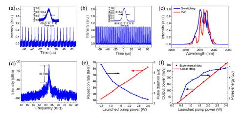
**Figure 4.** (**a**) Pulse series and monopulse waveform (inset) are 489.3 mW and (**b**) 2.99 W, respectively, at the power of the transmitting pump. (**c**) The measured spectrum of the pulse. (**d**) The RF spectrum of the pulse. (**e**) Change curve of launched pump power with repetition rate. (**f**) Launched pump power change curve with output power [205]. Copyright 2016 Nature Publishing Group.
