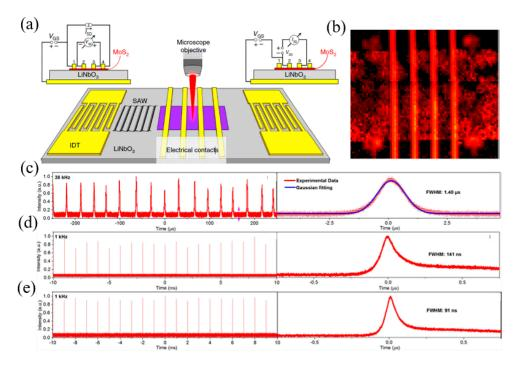
**Figure 17.** (a) Schematic diagram of device based on MoS<sub>2</sub>/LiNbO<sub>3</sub> combination. (b) PL map of the active FET region [292]. Copyright 2015 Nature Publishing Group. (c) Pulse trains of lasers and single pulses of WS<sub>2</sub> Q-switched. (d) AOM&WS<sub>2</sub> Q-switched at 1 kHz. (e) AOM&WS<sub>2</sub> based Q-switching at 1 kHz [293].
