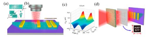
**Figure 30.** (a) The crystal structure imaging of Te, and wherein three atoms form a chain. (b) Schematic diagram of Te PD. (c) The net polarized photo-generated current  $\Delta$ Ip when the band of incident light is 2.3 µm in ambient temperature, and the incident power is 6.0 mW. (d) Infrared imaging method structure diagram [160]. Copyright 2020 Nature Publishing Group.
