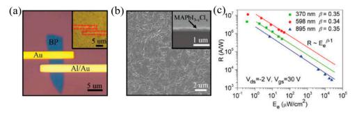
**Figure 24.** (a) Image of a BP/MAPbI<sub>3-X</sub>Cl<sub>X</sub> Schottky FET. The inset figure exhibits decorated with MAPbI<sub>3-X</sub>Cl<sub>X</sub> perovskite. (b) A typical plane view SEM image of the MAPbI<sub>3-X</sub>Cl<sub>X</sub> perovskite on silicon substrate. The inset figure shows the corresponding cross-sectional SEM image. (c) The response rate increases with the decrease in light intensity [313]. Copyright 2019 Wiley-VCH Verlag.
