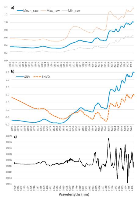
**Figure 1.** (a) Average (bold line), maximum and minimum (thin lines) of raw NIR spectra. (b) Standard normal variate (SNV) and standard normal variate plus detrending (SNVD) pre-treatments. (c) SNVD and first-order derivative pre-treatments. Spectra were recorded as log(1/R).
