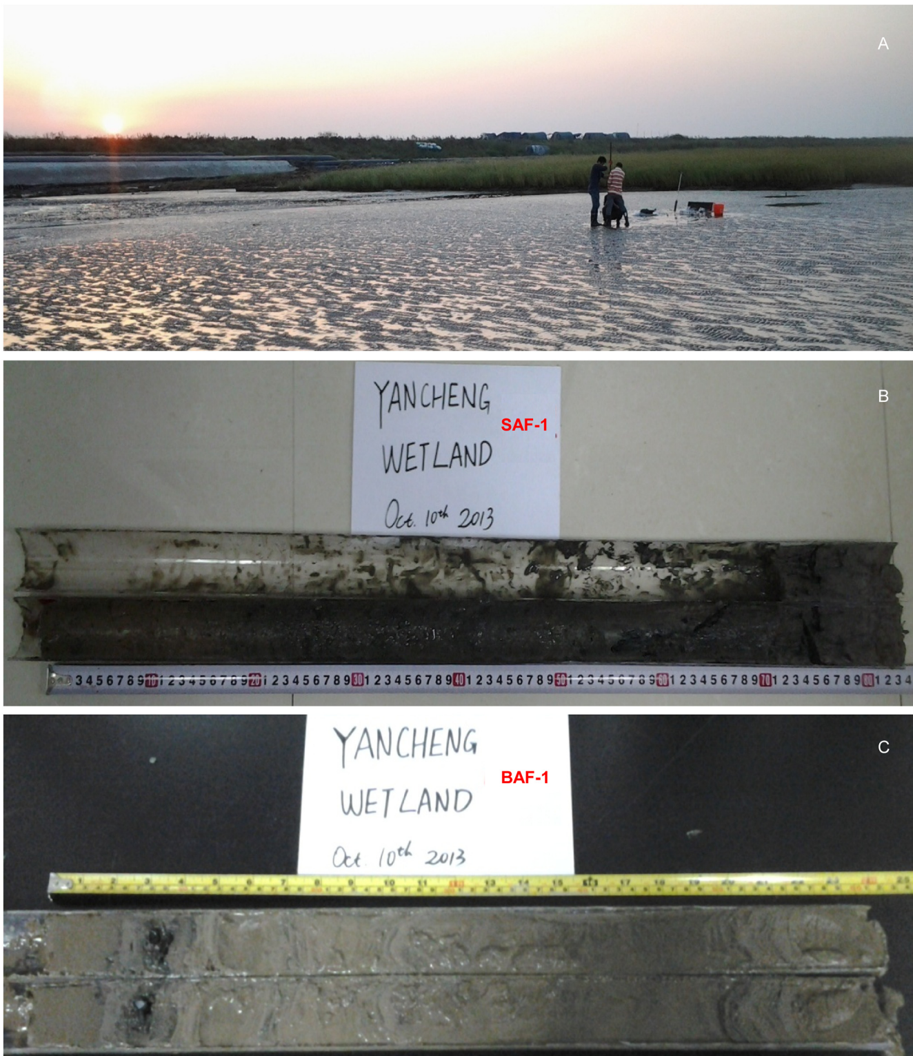
Fig 2. Photos of core sampling. (A) A photo showing the sampling site scene at Yancheng coastal wetland and core sampling in the field. (B) and (C) Photos showing the sediment cores of SAF-1 and BAF-1. PVC pipes were cut in half to show the lithologic character in the laboratory.
