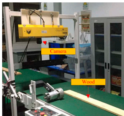
Figure 12. Wood image acquisition equipment.
