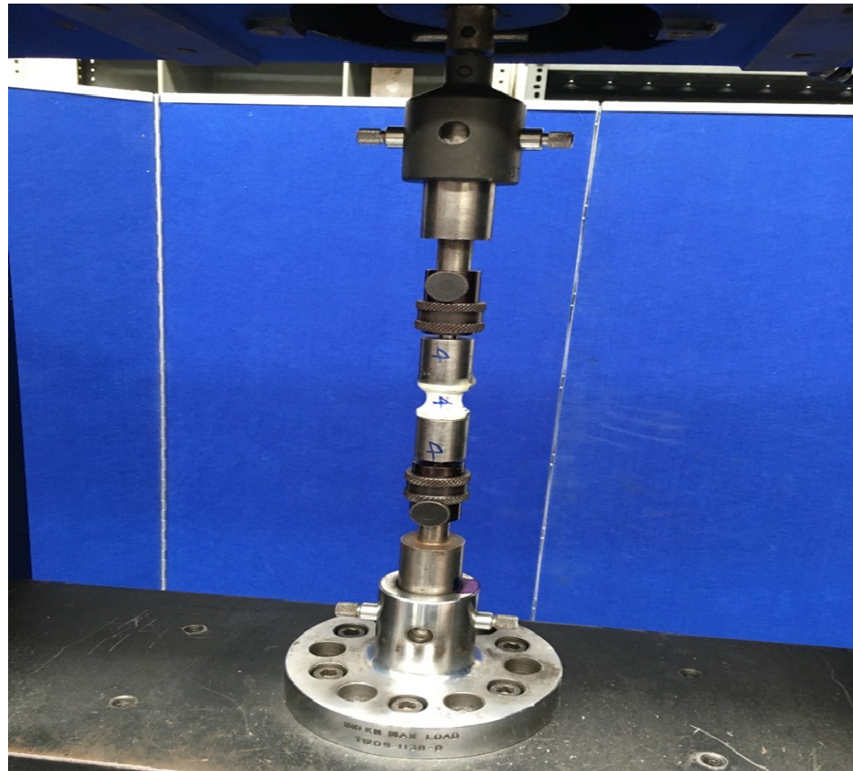
Figure 4. Through-thickness sample during testing in the tensile machine.
