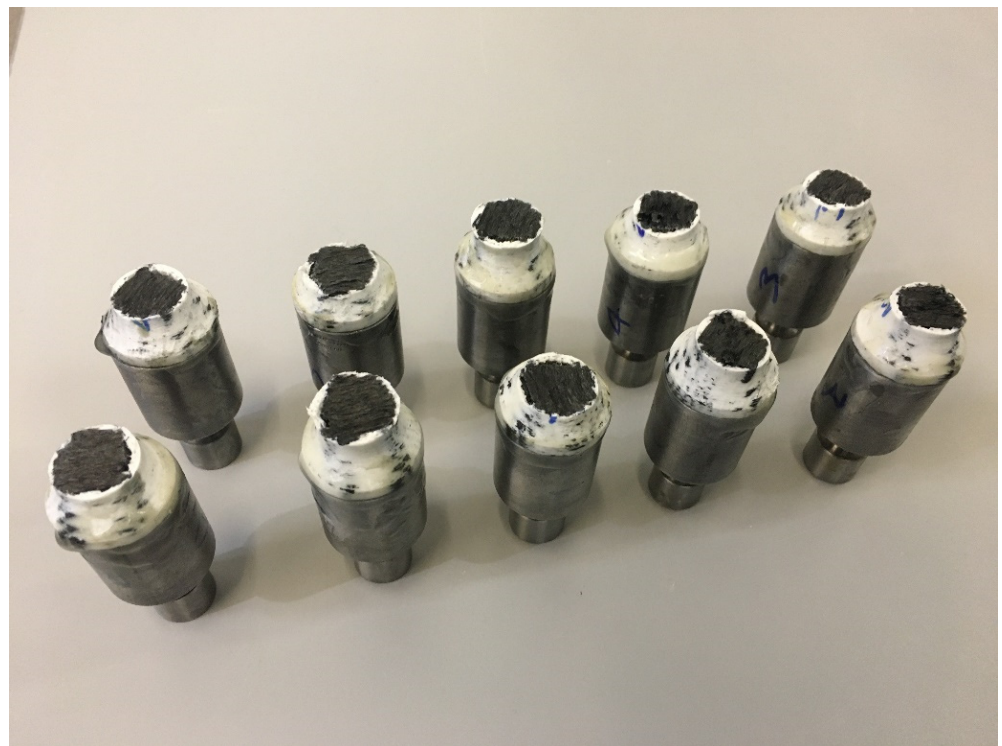
Figure 5. Fracture samples after testing with a consistent failure region.
