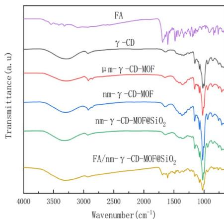
Fig. 2 FTIR spectra of FA,  $\gamma$ -CD,  $\mu$ m- $\gamma$ -CD-MOF, nm- $\gamma$ -CD-MOF, nm- $\gamma$ -CD-MOF@SiO<sub>2</sub>, FA/CD-MOF@SiO<sub>2</sub>.
