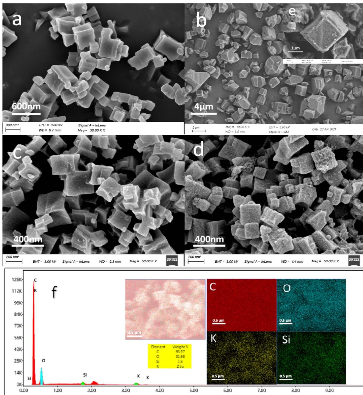
Fig. 1 SEM images of (a) nm-CD-MOF, (b)  $\mu$ m-CD-MOF, (c) nm-CD-MOF@SiO<sub>2</sub>, (d) FA/nm-CD-MOF@SiO<sub>2</sub>, (e)  $\mu$ m-CD-MOF@SiO<sub>2</sub>, (f) EDX mapping for nm-CD-MOF@SiO<sub>2</sub>.
