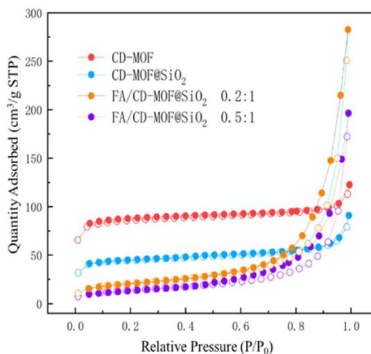
Fig. 4 N<sub>2</sub> adsorption-desorption curve for CD-MOF, CD-MOF@SiO<sub>2</sub> and FA/CD-MOF@SiO<sub>2</sub>.
