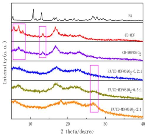
Fig. 5 XRD pattern of FA, CD-MOF, CD-MOF@SiO<sub>2</sub> and FA/CD-MOF@SiO<sub>2</sub>.
