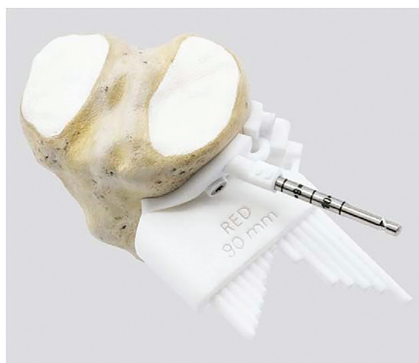
Figure 5. Drill guide shown with an additional drill depth limit clipped onto the drill guide. The drill depth limiter has cannulated sleeves through which a length-standardized drill bit is passed. The length of these cannulated sleeves creates a hard stop for the drill, preventing overpenetration with drill bits.
