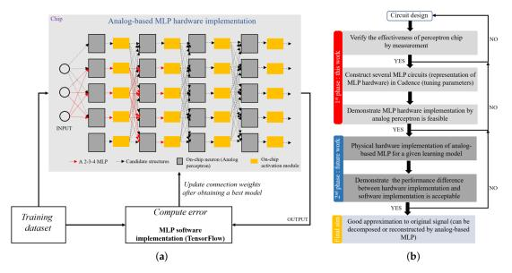
**Figure 2.** (a) Configuration of our proposed analog-based MLP and learning algorithm. (b) Contributions in this work.
