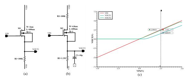
**Figure 8.** Circuits and simulation for the rectified linear unit (ReLU) activation function. (**a**) A source follower circuit. (**b**) Our improved source follower circuit. (**c**) Simulation results for both circuits.
