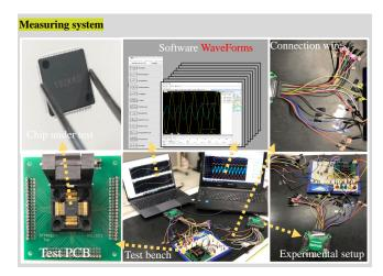
Figure 3. The general architecture of the measuring system for the perceptron chip.
