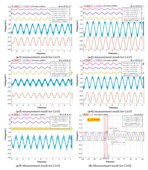
Figure 6. Measurement results for perceptron chip.
