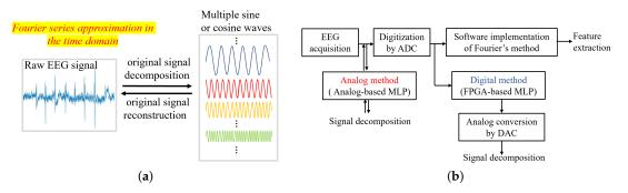
**Figure 1.** Comparison between the analog method and digital method aimed at electroencephalogram (EEG) signal processing with machine learning mechanism. (**a**) EEG signal decomposition/reconstruction by using fourier series approximation. (**b**) The analog-based multi-layer perceptron (MLP) and field programmable gate array (FPGA)-based MLP in the handling of the EEG signal.
