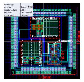
Figure 5. Top-level layout of perceptron chip.
