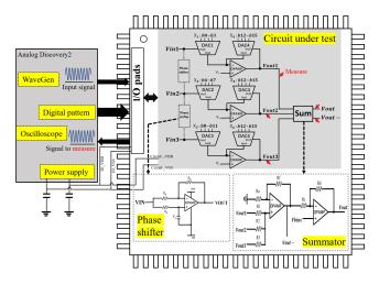
Figure 4. A schematic of a perceptron chip and block diagram of the measurement.
