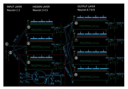
Figure 7. Top-level schematic of our MLP circuit.
