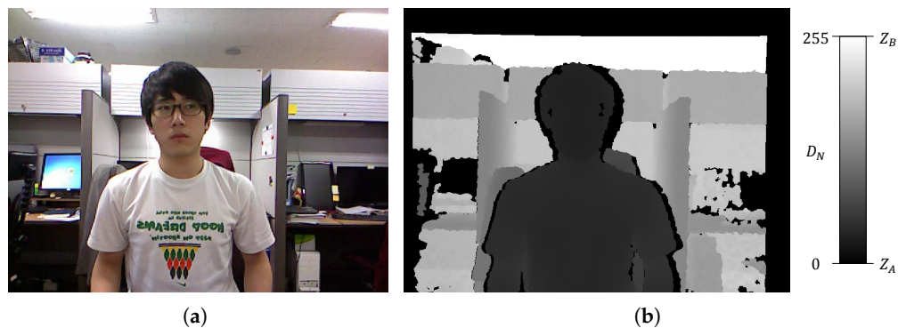
Figure 3. Aligned (a) color and (b) depth image pair. The depth images are normalized to D_N (between 0 and 255).
