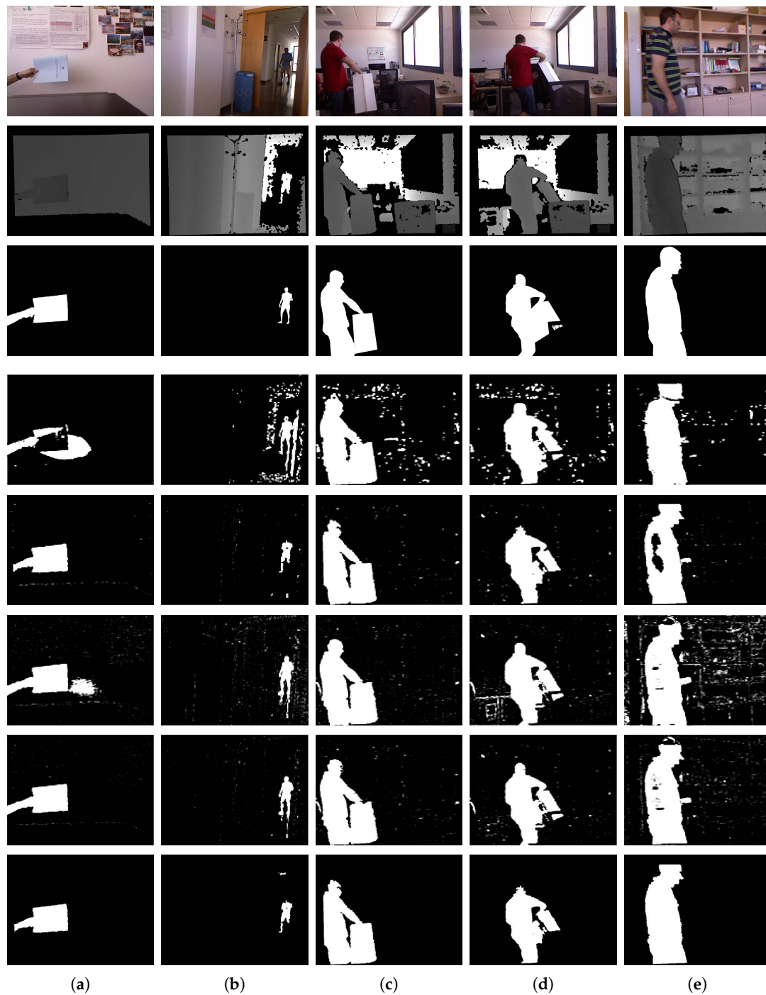
Figure 10. Experimental results using Fernandez's Kinect dataset ((a–e) indicate Wall #93; Hallway #120; Chair Box #278, #286; Shelves #197, respectively). Rows 1–3 are the color images, depth images, and ground truth, respectively. Rows 4–8 present the results given by MOG4D, CB1D, CB4D, DECB, and the proposed method, respectively.
