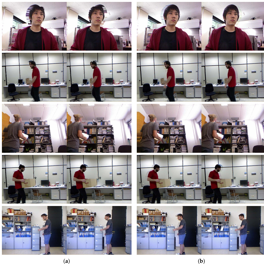
Figure 17. Comparison of the quality of the stereoscopic images. (a,b) are generated using original and enhanced depth images by the proposed method, respectively.
