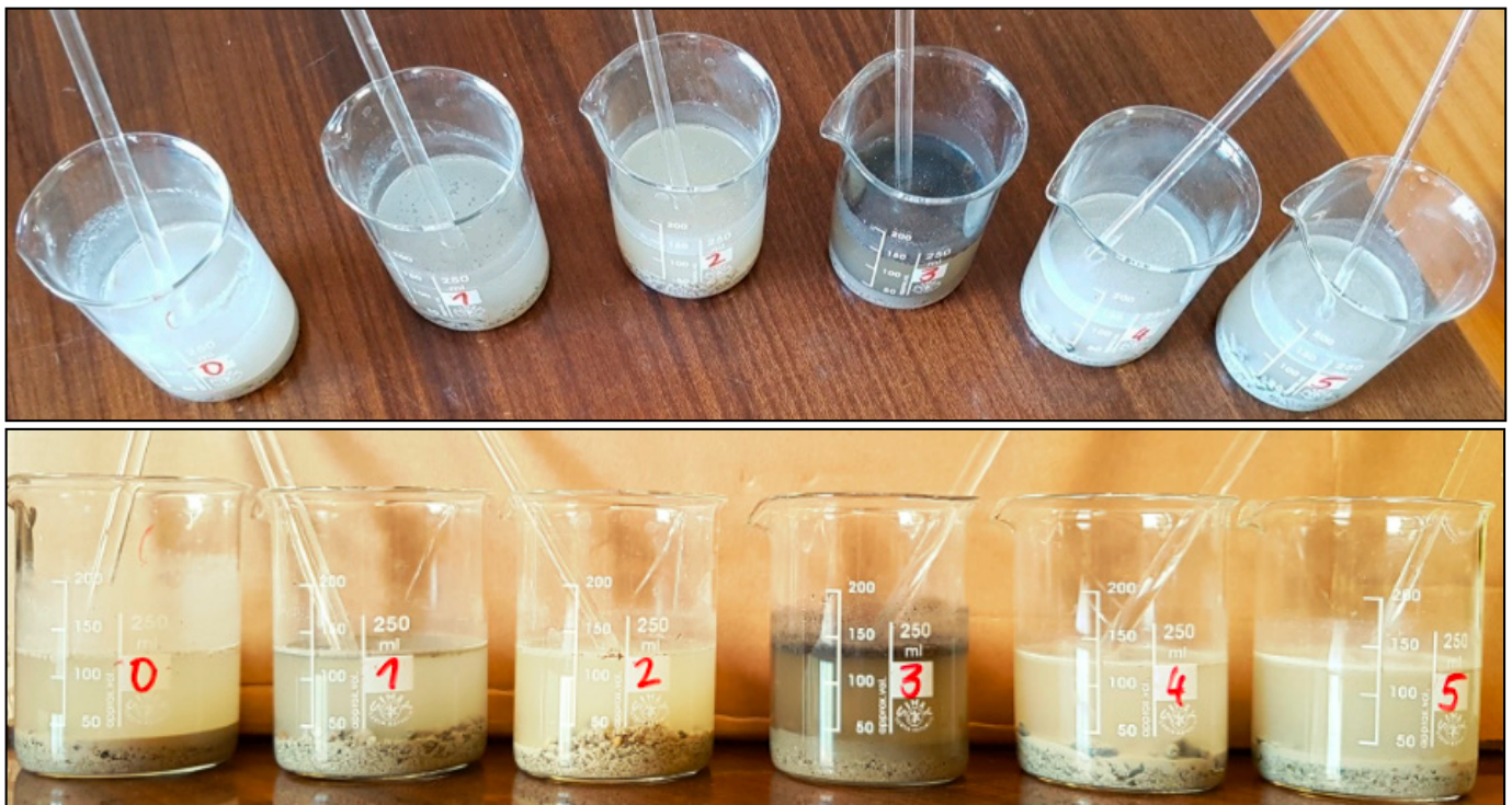
Figure 10. Suspensions made from deionized water and crushed concrete from the bridge.
