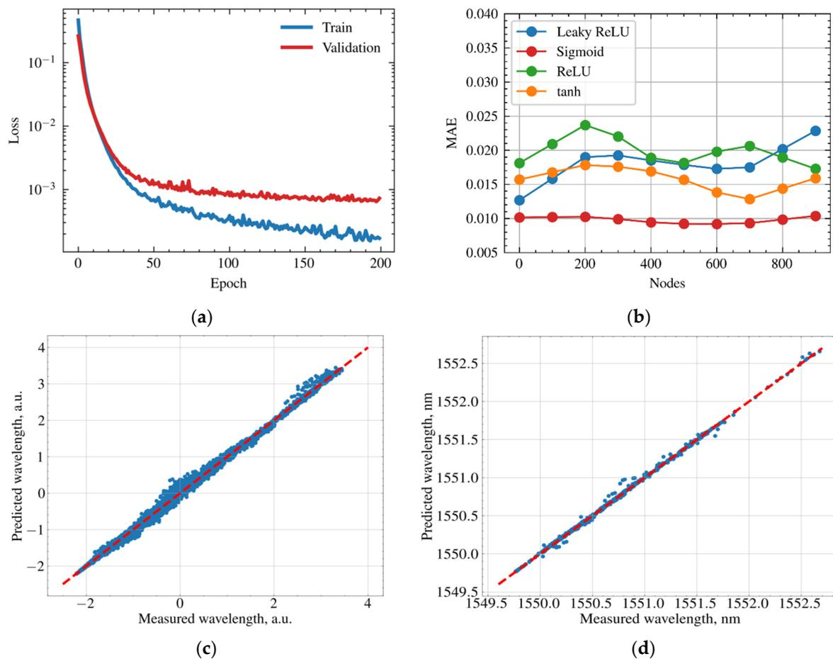
**Figure 9.** Performance of the CNN (a) Learning curve of the model on training dataset and evolution of the loss function of validation dataset. (b) Mean absolute error of CNN for different activation functions and different number of nodes of the fully connected layers. (c) Predicted reflectance peak positions of the FBGs of the sparse sensors against measured values at normalized scales. (d) Predicted positions of the reflectance peak for single FBG of sparse sensor against measured value.
