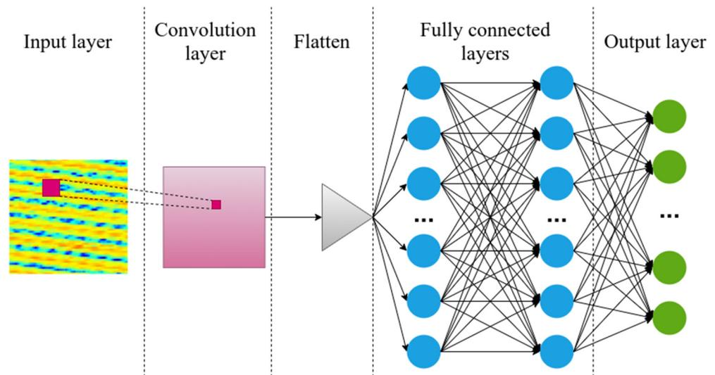
**Figure 6.** Convolutional neural network consisted of six layers.
