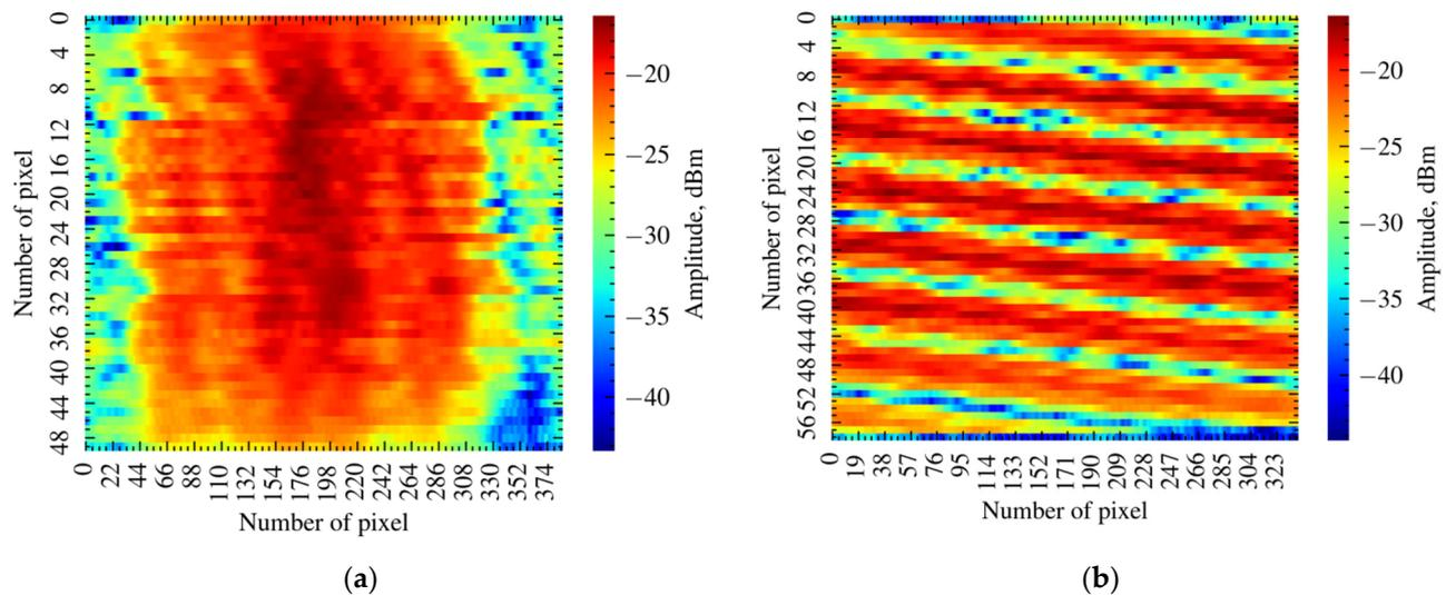
**Figure 7.** (a) 2D reflectance spectrum of FBG sensor with centered reflectance peaks; (b) 2D reflectance pattern of FBG obtained by slicing the reflectance spectrum into 59 pieces.
