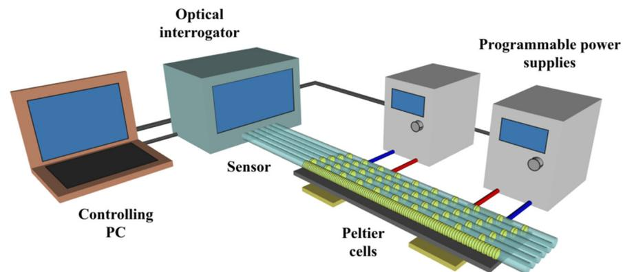
Figure 3. Principle scheme of the experimental setup.
