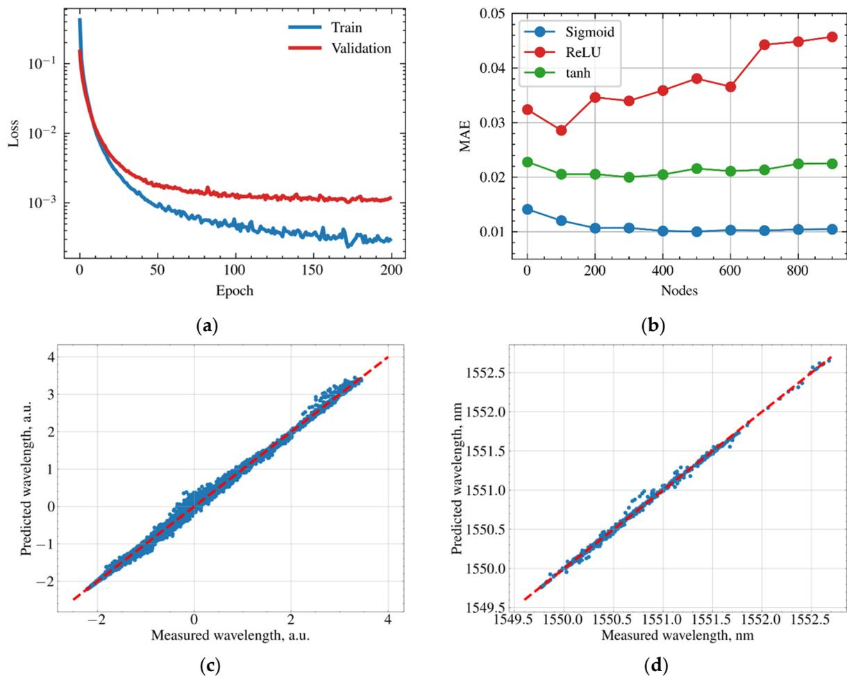
**Figure 8.** Performance of the FCNN. (a) Learning curve of the model on training dataset and evolution of the loss function of validation dataset. (b) Mean absolute error of FCNN for different activation functions and different number of nodes of the hidden layer. (c) Predicted reflectance peak positions of the FBGs of the sparse sensors against measured values at normalized scales. (d) Predicted positions of the reflectance peak for single FBG of sparse sensor against measured value.
