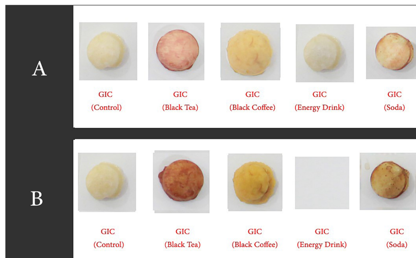
Fig. 4 GIC Specimens ready for measurements. A GIC (after 2 weeks). B GIC (after 4 weeks).
