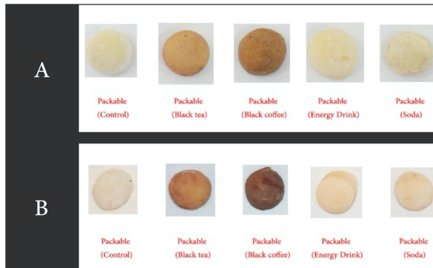
Fig. 3 Composite Specimens ready for measurements. A Composite resin (after 2 weeks). B Composites resin (after 4 weeks).
