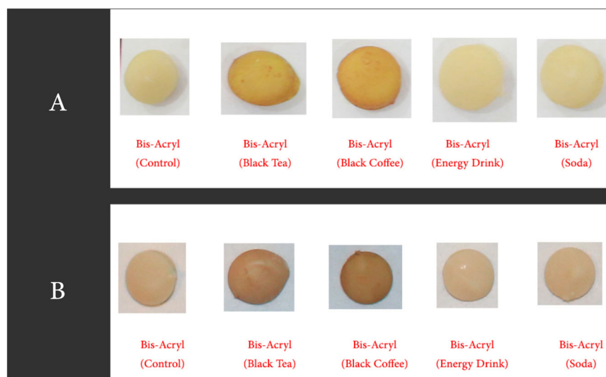
Fig. 5 Bis-acryl Specimens ready for measurements. A Bis-acryl (after 2 weeks). B Bis-acryl (after 4 weeks).
