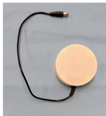
Figure 1. The spinning permanent magnet (SPM) device.
