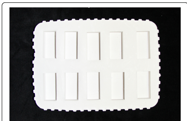
Fig. 2 Mold used for vulcanization of white-group samples
