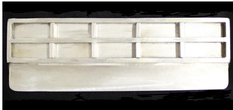
Fig. 3 Stainless steel mold fabricated to vulcanize control group samples
