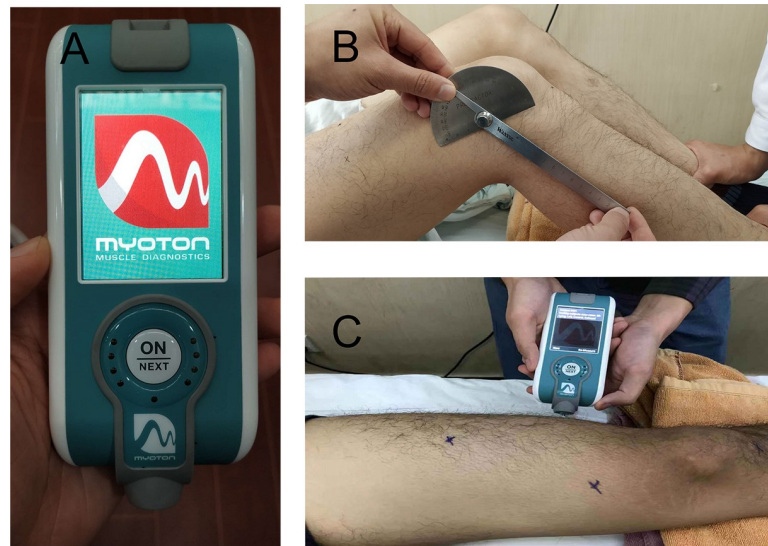
Fig 1. The MyotonPRO measurement technique. (A) MyotonPRO device; (B) Identification of measurement angle; (C) Measurement with MyotonPRO.
