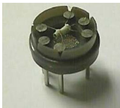
Figure 2. Taguchi chemoresistive gas sensor. Reprinted with permission from Ref. [38]. Copyright 2015, Neri, G.
