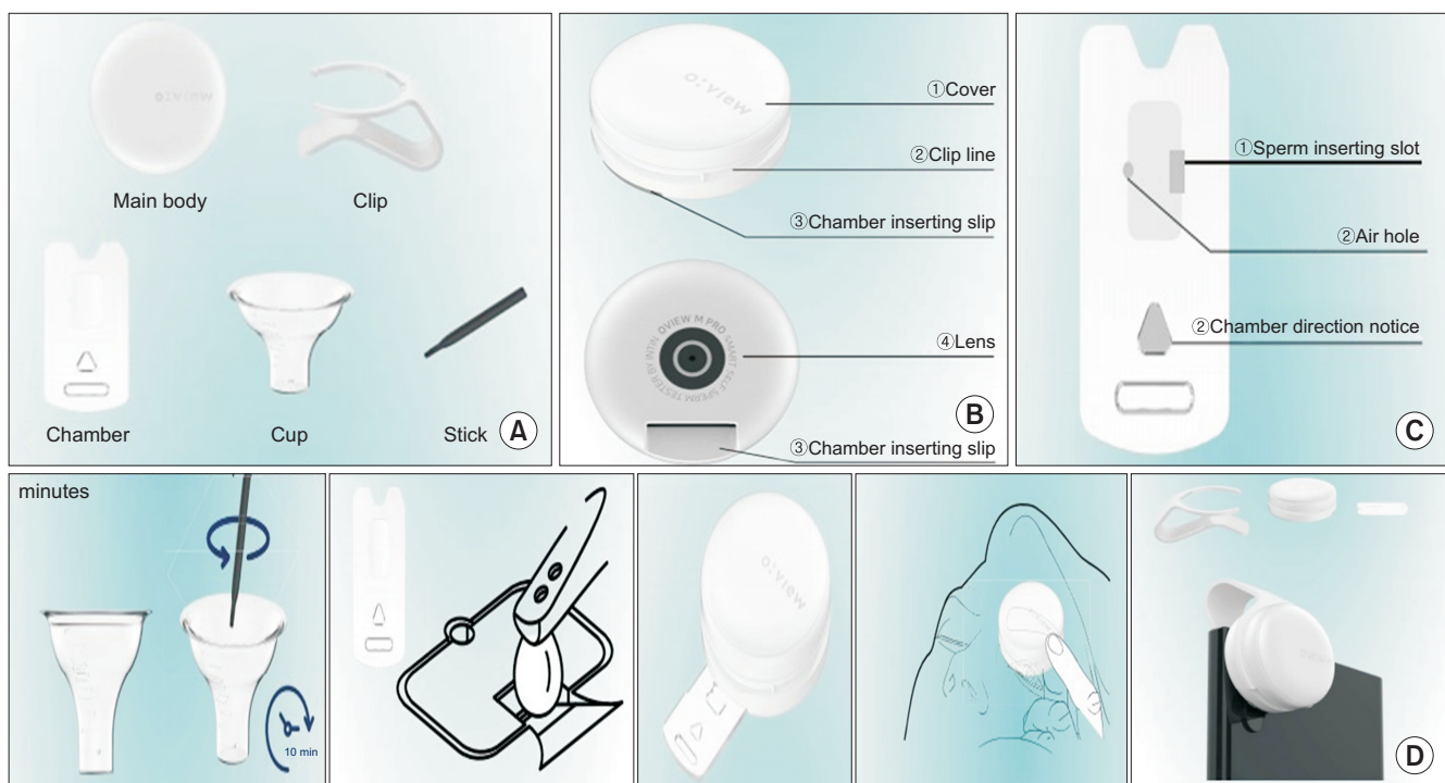
Fig. 1. Device and components of O'VIEW-M PRO ® system. (A) Components of O'VIEW-M PRO ® is consisted of main body with clip, chamber, semen cup, and stick. (B) Main body is consisted of cover, clip line, chamber inserting slip, lens, and built-in LED light source. (C) The liquefied semen sample is dropped into the sperm inserting slot. (D) Assay procedure with smartphone-based App assisted semen analysis, O'VIEW-M PRO ® . After semen collection, liquefaction and stirring, semen loaded on 0.05 mL (1 drop) in the sperm inserting square slot of chamber and insert the chamber into the chamber inserting slip of main body. Sperm can be observed through the lens of main body by the naked eye. After fixing the attachment of the lens and body of the smartphone with a clip, the sample test result with concentration and mobility is shown as a screenshot.
