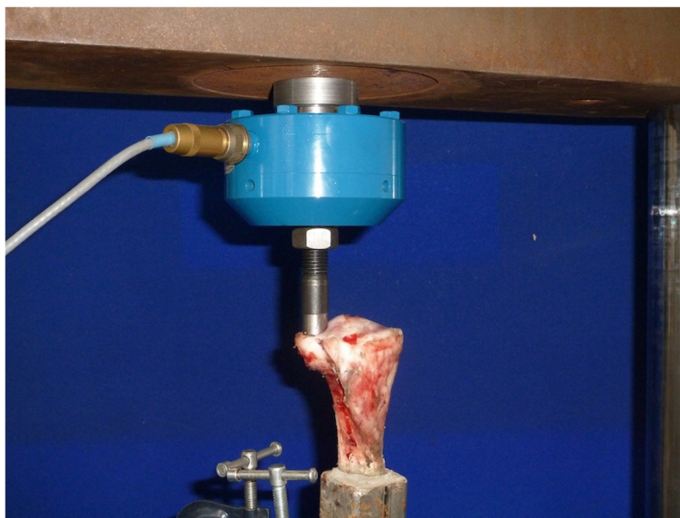
Figure 2 Digital photograph showing a specimen mounted on hydraulic compression testing machine.
