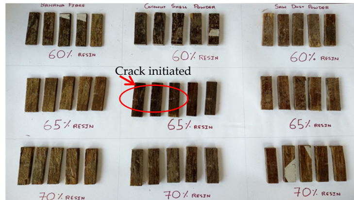
Figure 5. SENB test specimens.
