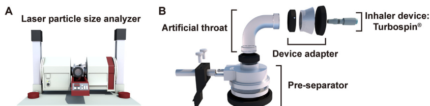
Figure 2 Schematic diagrams of MPAP (A) Laser particle size analyzer; (B) Changeable module.
