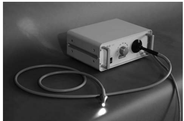
Fig. 2. Broadband NIR emitter. An ear speculum at the end of the fibre-optic cable aids in the application of NIR radiation in the auditory canal.
